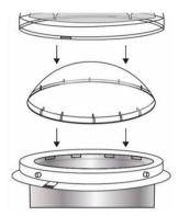
Snap the dome onto the dome ring using the 4 snap closures. Ensure that all four connecting points are properly engaged.
