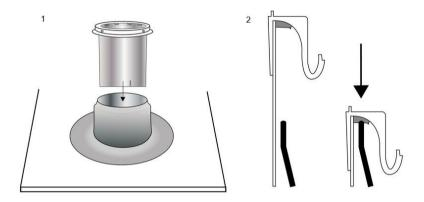
Fix the dome ring onto the top of the flashing with the dome screws, screwed through the four grey spacers from the outside in. The screws will pierce through the flashing and the inside of the reflective tubing. Be careful not to overtighten the screws as this may cause damage to the dome ring.
