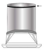
Push the end of the tube with the brush sealing strip applied up through the ceiling opening and up into the top tube assembly. Slide the tube from below through the recess in the ceiling.
