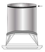
Push the end of the tube with the brush sealing strip applied up through the ceiling opening and up into the top tube assembly. Slide the tube from below through the recess in the ceiling.
