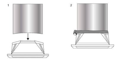
ECO version - Fit the insulating lens onto the top of the bottom tube assembly and tape the outer edge of the lens to the outside of the tube with aluminium tape.
