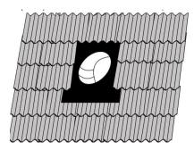
The three tile clips provided are also used to secure the bottom skirt of the flashing down onto the roof. Clamp the short "leg" of the clips between two tiles beneath the edge of the flashing and bend the long "leg" back over the edge of the flashing to clamp it in place.
