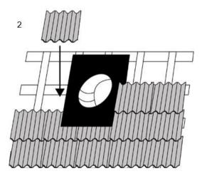
Secure the lower skirt of the flashing down onto the tiles below with the High-tack adhesive / sealant and tile clips provided.
