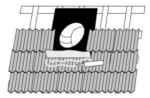
Fit the roof tiles back around the sides and top of the roof flashing.
