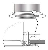
Now remove the transparent protective film from the inside of the bottom tube assembly.
