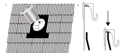
Fix the dome ring onto the roof flashing using the dome screws provided, screwed through the four grey spacers from the outside in. The screws will pierce through the flashing and the inside of the reflective tubing. Be careful not to overtighten the screws as this may cause damage to the dome ring.
