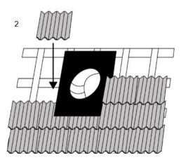
Secure the lower skirt of the flashing down onto the tiles below with the High-tack adhesive / sealant and tile clips provided.
