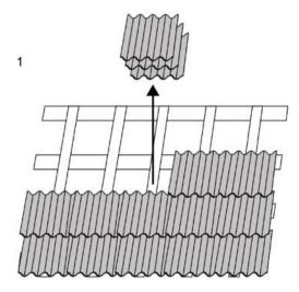
Determine the ideal position so that the flashing can be installed beneath the tiles above / to the sides and down onto the tiles below.
