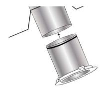
**Tip:** Make sure that the mounting clips on the ceiling ring are in a 'closed' position so that they fit through the ceiling opening.
