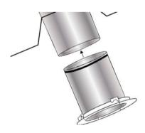
**Tip:** Make sure that the mounting clips on the ceiling ring are in a 'closed' position so that they fit through the ceiling opening.
